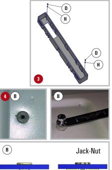
Warning: Before drilling into the truck floor make sure the area where you are going to drill through is clear of any electrical wiring, fuel lines, tanks, and reservoirs. You will have to look under the vehicle to make sure there are no obstructions at the hole locations.
