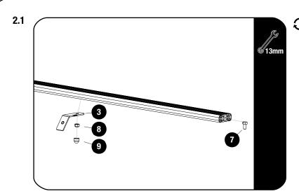
Slide one M8 x 16 Hex Head Bolt (Item 7) into the T-slot of the front slat. Center the mid support bracket in the middle of the slat and secure using M8 Nyloc Nut (Item 8). Fully tighten.
