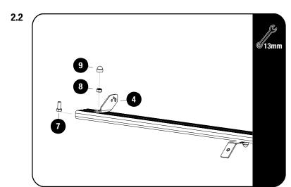
Fit the Light Bar Bracket 01 LH / RH (Item 4) for for the 40" Light Bar, using M8x16 Hex Bolt & M8 Nyloc Nut (Items 7 & 8). Fit the light bar and center it on the slat before fully tightening the brackets.
