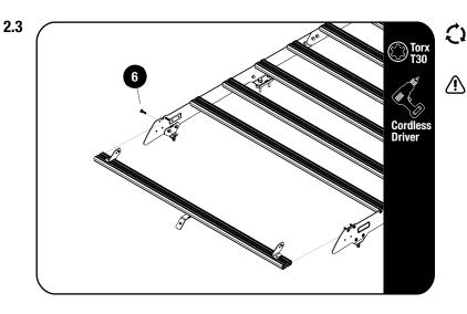
Secure assembly 2.2 to the front two top holes on the foot rails using the fasteners supplied with KSTF001.
