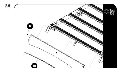
Fit the Wind Fairing Rubber (Item 10) to the Light Bar Wind Fairing (Item 1). Using the notched section as a guide, trim if needed.
