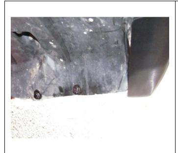
166. Mark and drill 2 x Ø7mm holes through each of the inner guards in line with the cage nuts.
