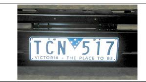
176. Fit the plastic plugs into the square holes in the lower pan. Fit the number plate to the bull bar using the black self-tapping screws.
