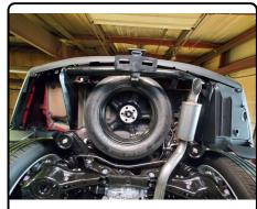
7. Mark and trim underbody panel. Reattach muffler lowered in Step (5) and underbody panel using fasteners removed in Step (1).
