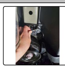
5. Lower muffler by removing exhaust hanger rod closest to the exhaust tip from rubber isolator. Reinstall in STEP 7.
