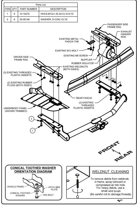
1. Remove the (7) fasteners securing the driver side underbody panel. After lowering the underbody panel return it to the owner or trim and reinstall in Step (7).
