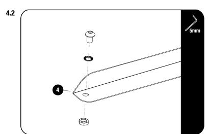
Loosely assemble the M8 x 12 Button Head Bolt, M8 Schnorr Washers and M8 Thin Nut both LH & RH Wind Deflectors (Item 5) as shown.
