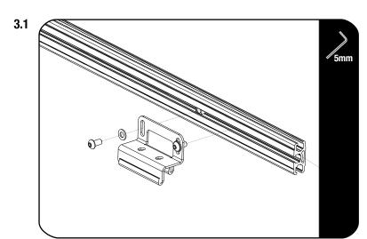
Loosely assemble the FPCR Feet (Item 7) using M8 x 16 Button Head Bolts, M8 Flat Washers and M8 Nyloc Nuts and slide them into the side profiles. They must still be able to slide freely.
